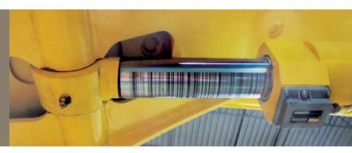
built in by utilising two or more sensors mounted around a piston rod with full radial marking, providing improved redundancy over other linear sensing devices.
